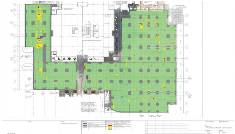
Figure 9: On-site GPR corrosion results.
