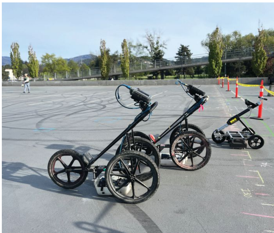
Figure 2: Ground-penetrating radar (GPR) and objective acoustic sounding system.
