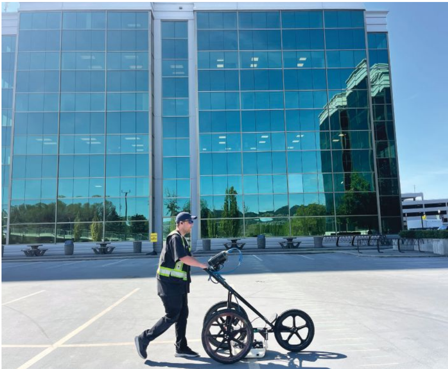
Figure 4: On-site GPR survey.
