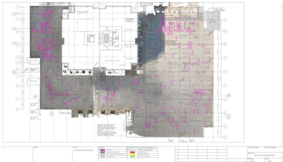
Figure 10: On-site sounding delamination results.
