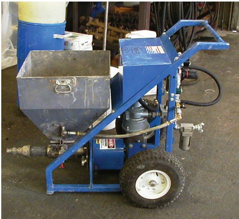
Fig. 10: Small wet spray machine, larger models available
