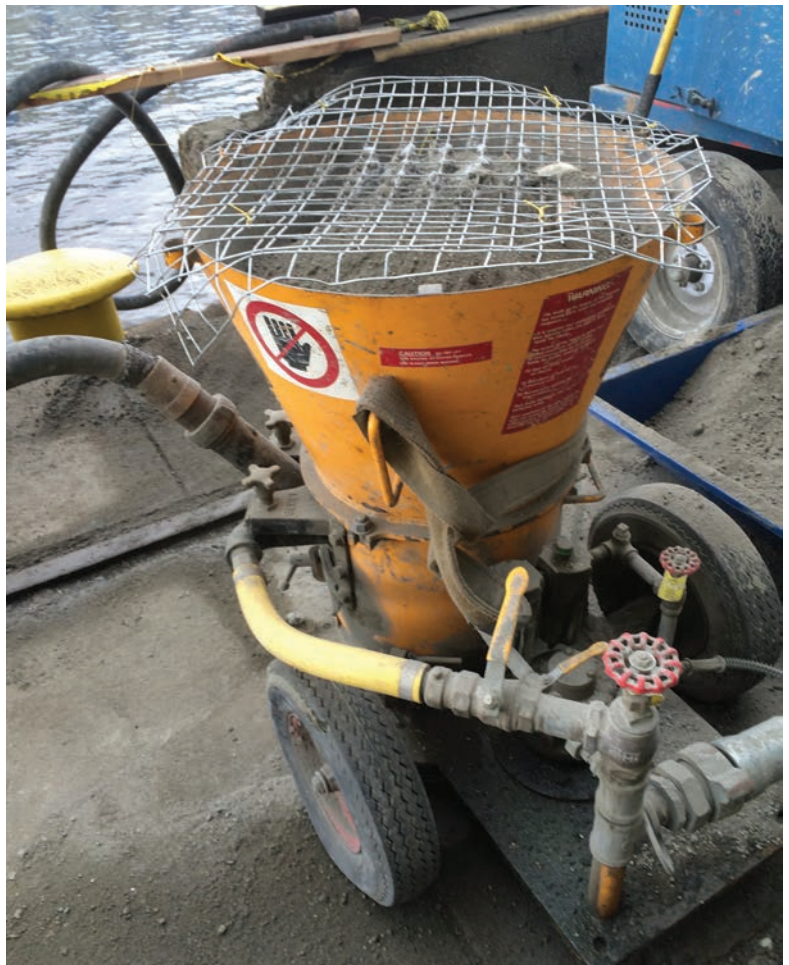
Fig. 7: Dry process shotcrete rig: compact, yet capable of significant application rates
