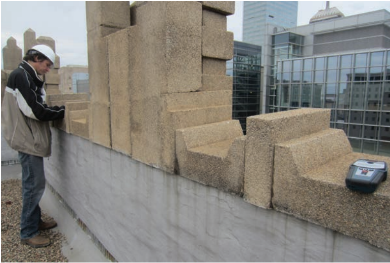
Fig. 4: Measurements were made of the brick and cast stone capitals
