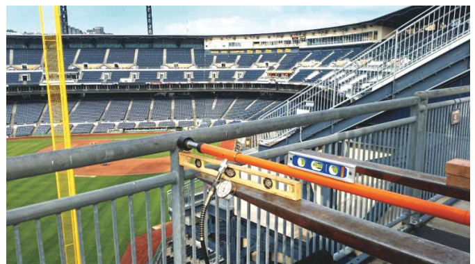
Fig. 4: Load testing of typical handrail
