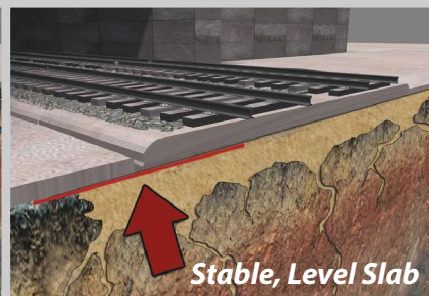
Injecting Lifting Foam
