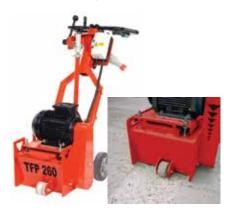
The TFP 260 has a 10" cutting width and 1/4" maximum cutting depth per pass. Depth control enables removal of surface materials without damaging the substrate, maximizing performance and extending cutter life. Other features include a quick-lift drum lever for operator control and integrated vacuum connection for dust-free scarifying.
