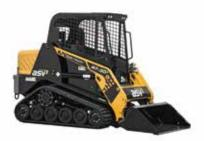
The 3,600-pound RT-30 is 48 inches wide and has an 8.4-foot lift height. Its compact size and 10 inches of ground clearance minimize risk of property damage or damage to the machine while working in hard-to-reach areas, whether clearing snow on sidewalks and through alleys or while completing landscaping or construction work in high-density housing areas.
