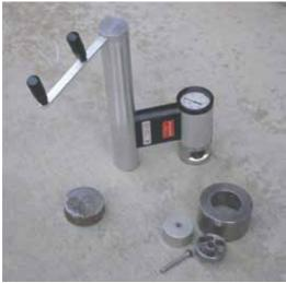
Fig. 2: Pull-off bond testing equipment
