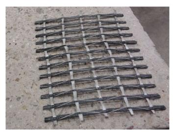
Fig. 2: Unidirectional carbon grid
