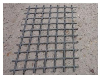
Fig. 3: Bidirectional carbon grid
