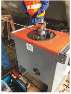
Fig. 8: Titanium bar bending onsite: (a) Cutting bar to length with abrasive saw; (b) Heating bar with a torch; (c) Bending bar with hydraulic rebar bender
