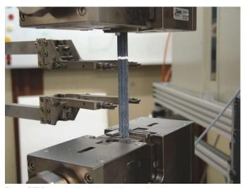
Fig. 4: CFRP sample after failure during tensile stress test
