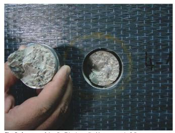
Fig. 9: A successful pull-off test resulted in a concrete failure
