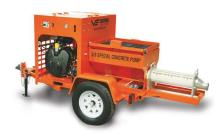
The 38 Special Concrete Grout Pump is available in a small trailer mounted unit which can easily be towed by a ½ ton truck as well as a skid mounted version. It has an 8 Cubic Foot Hopper with a 4-inch Heavy Duty Clamp Discharge to easily handle 3/8" aggregate pumpable mix designs. With pumping distances in excess of 200 Feet Horizontal and 80 Feet Vertical, the 38 Special can make impossible projects possible.
