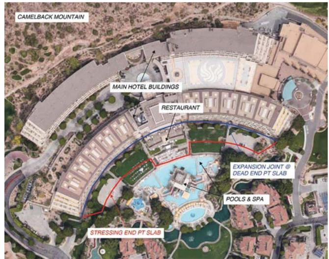
Fig. 2: Overhead view of subgrade garage
