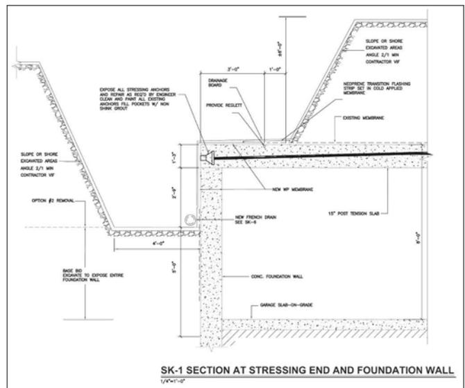
Fig. 4: Section detail at stressing end and foundation wall (repair drawing)
