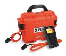
The third generation intelliRock system is the only concrete monitoring tool featuring profiling technology to allow users to detect delamination, monitor insulation performance, and view curing box and specimen temperatures and other temperature extremes. The system also delivers real-time information needed for safer and efficient management of concrete-related workflow.
