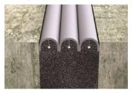
Willseal 250-R has no unbonded laminations. It allows for up to 100% (±50%) movement from mean joint size. Its advanced reinforced bellows provide 35 psi of point load resistance.
