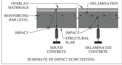
Fig. 4: Schematic of impact-echo testing
