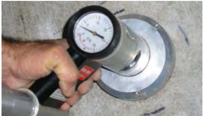
Fig. 1: Pulloff test on an overlay concrete (Fig. 7.2a from Reference 4) 7
