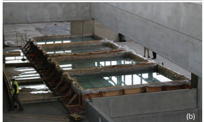
Fig. 4: Load test in progress: cyclic loading (a) and monotonic pool loading (b) (Images courtesy of Pivot Engineers)
