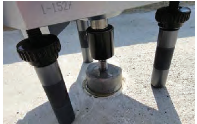
Fig. 2: Direct tension pulloff testing
