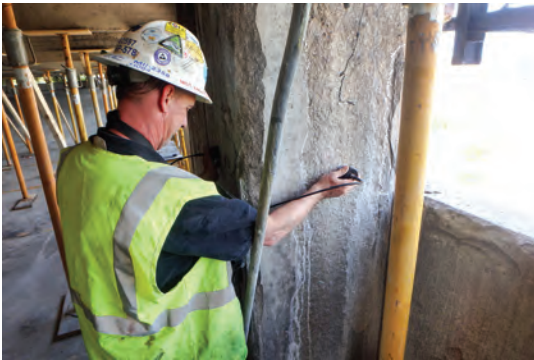
Fig. 5: Nondestructive testing performed at damaged column
