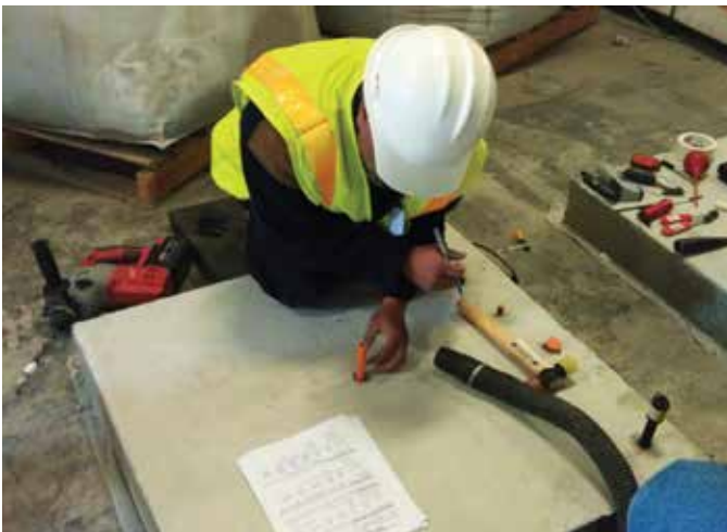
Fig. 3: Relative humidity (RH) testing being performed on test slab (photo courtesy of ICRI)
