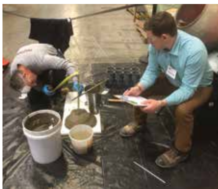
G&B Tile & Plaster President, Greg Musgrove, performing a concrete slump test
