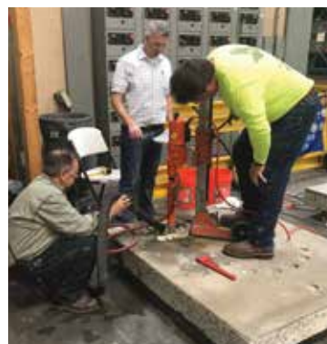
North Texas Treasurer, Pete Haveron, core-drilling an overlaid concrete slab under the watchful eye of CSRT judge, Jacob Borgerson
