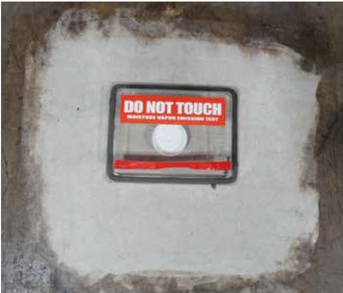
Fig. 2: MVER test in progress (photo courtesy of ICRI)
