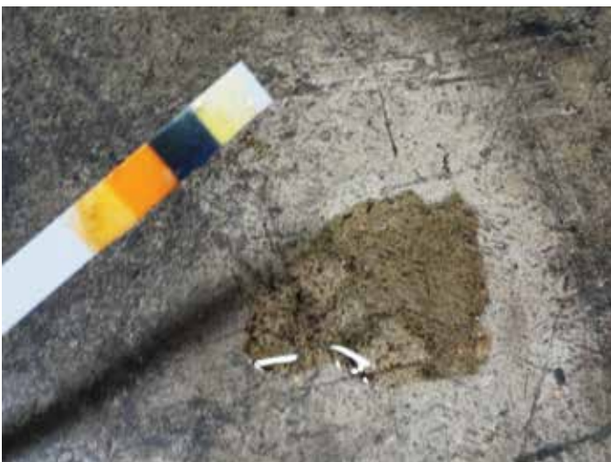
Fig. 4: pH testing using indicator paper (photo courtesy of ICRI)
