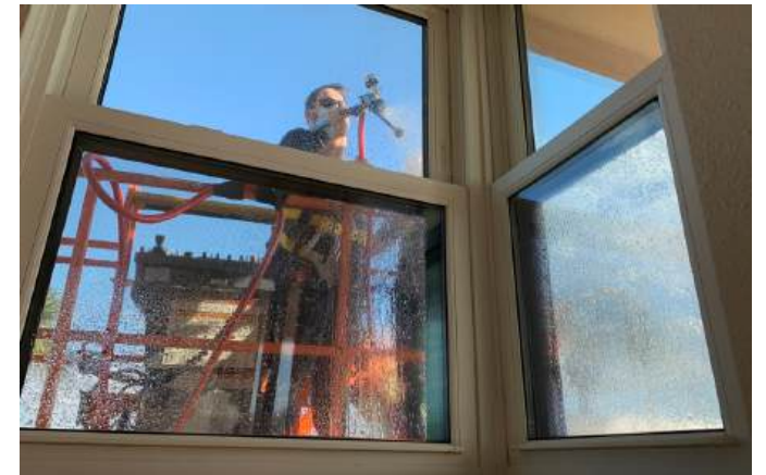
Fig. 3: Water testing at building exterior to replicate Hurricane Eta
