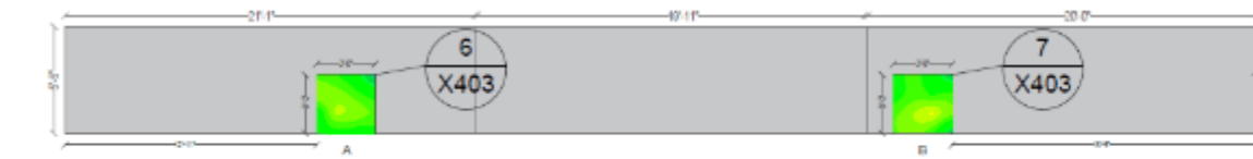
5 NORTH ELEVATION - CORROSION POTENTIALS (i-VOS) 3/16" = 1'-0"
