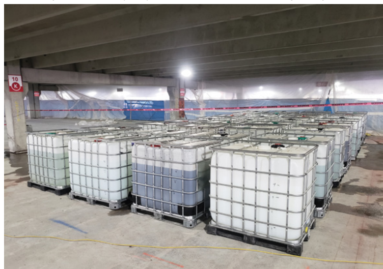
Load testing the slab to verify the performance of the new slab strengthening slots
