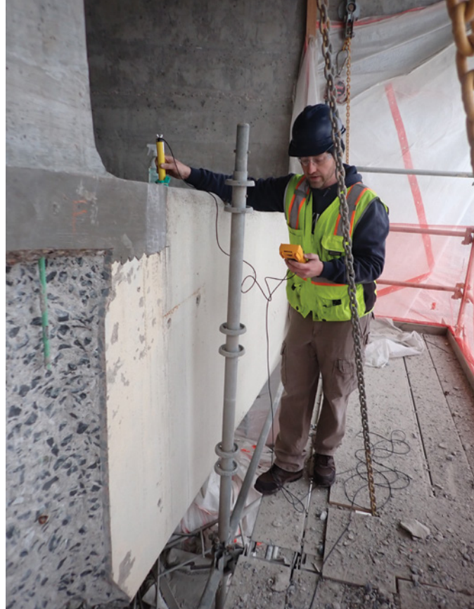
Image 10: Half-cell potential testing during construction
