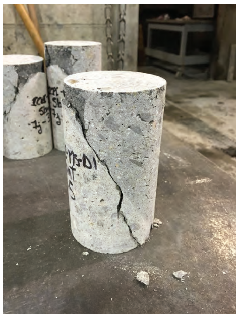
Fig. 6: Composite core for slant shear bond strength testing (ASTM C 882)
