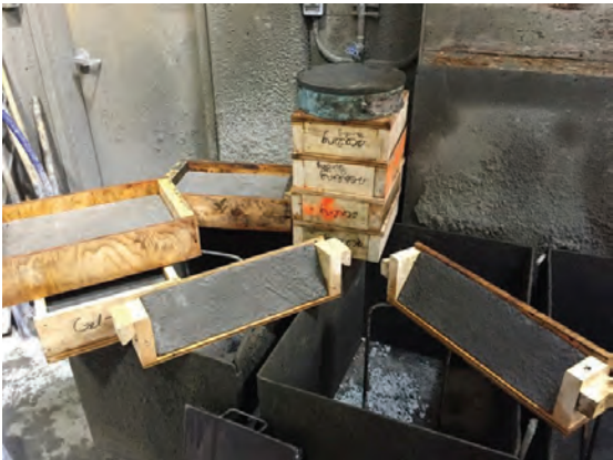
Fig. 5: Inclined precast mould for slant shear bond strength testing (ASTM C 882)
