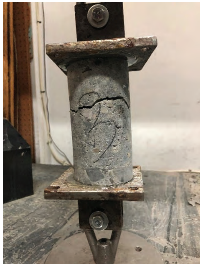
Fig. 12 Bond pull-off test at the laboratory
