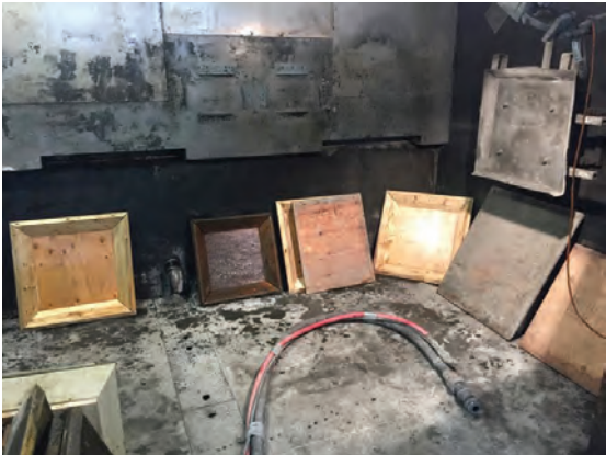
Fig. 3: Conventional square shotcrete test panels used for obtaining cores
