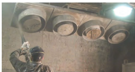
Fig. 8: Shotcrete being sprayed into inclined AASHTO T 344 rings
