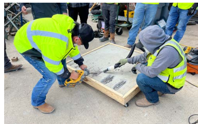
Fig. 4: Removing concrete from around reinforcing bars
