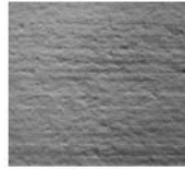
Fig. 6.4: CSP 4 (light scarification)
