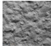
Fig. 6.7: CSP 7 (heavy abrasive blast)
