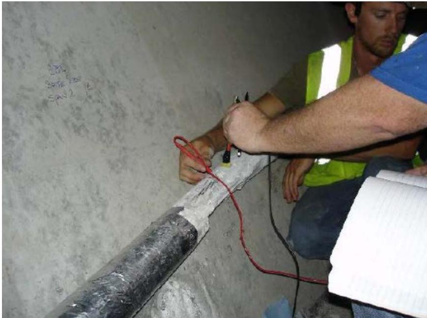
Table 4.2-2. Corrosion potential measurements.
