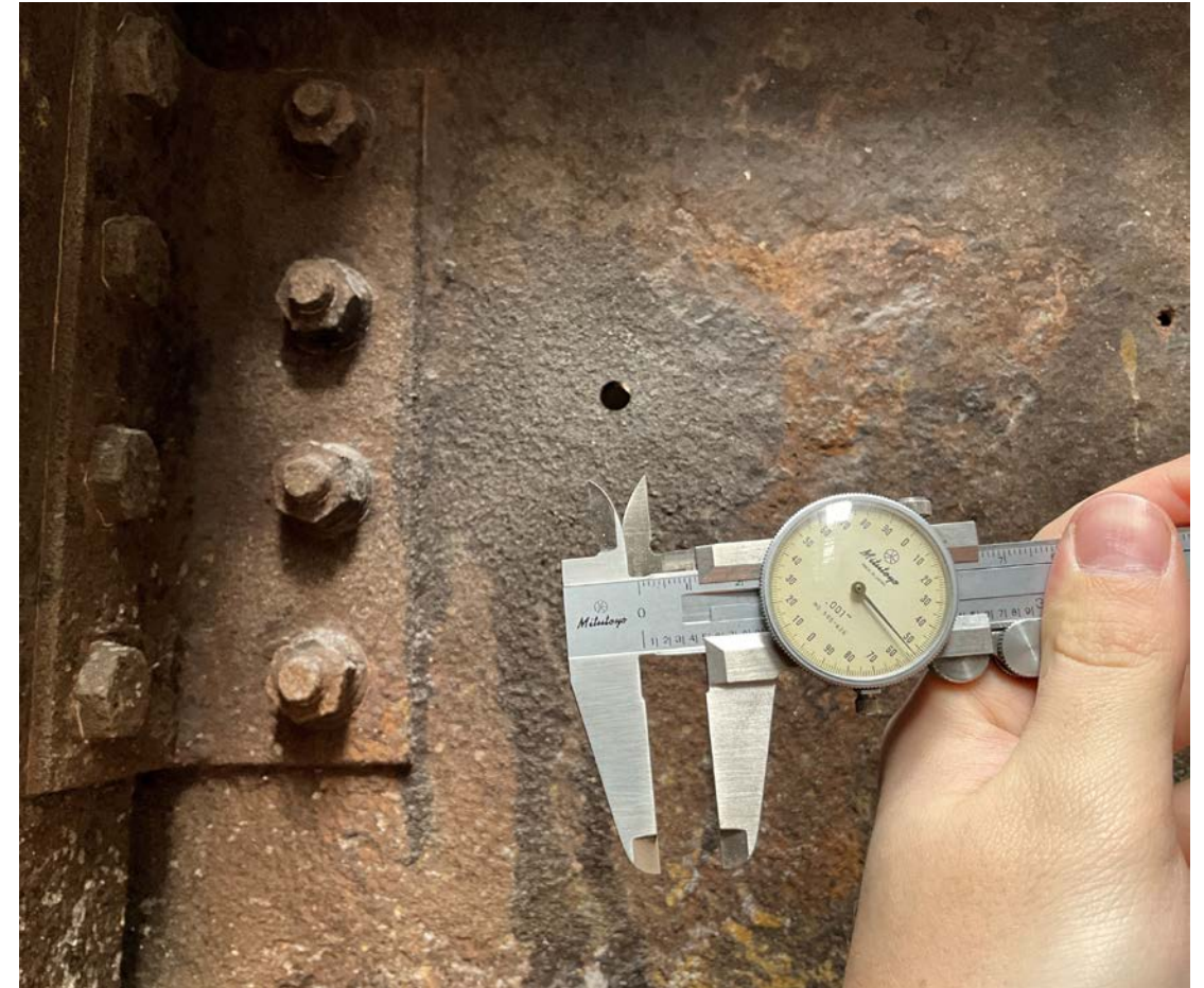
Calipers for measuring thicknesses
