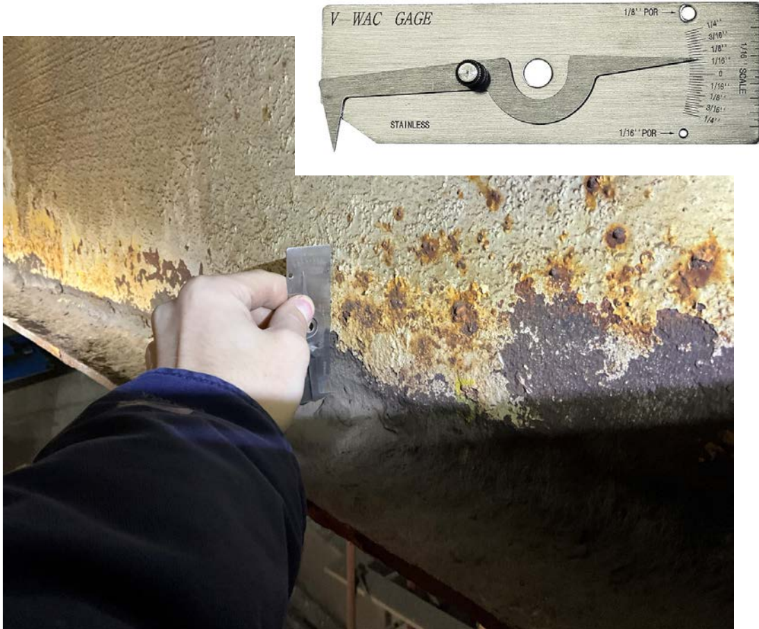
V-WAC gage for measuring pitting
