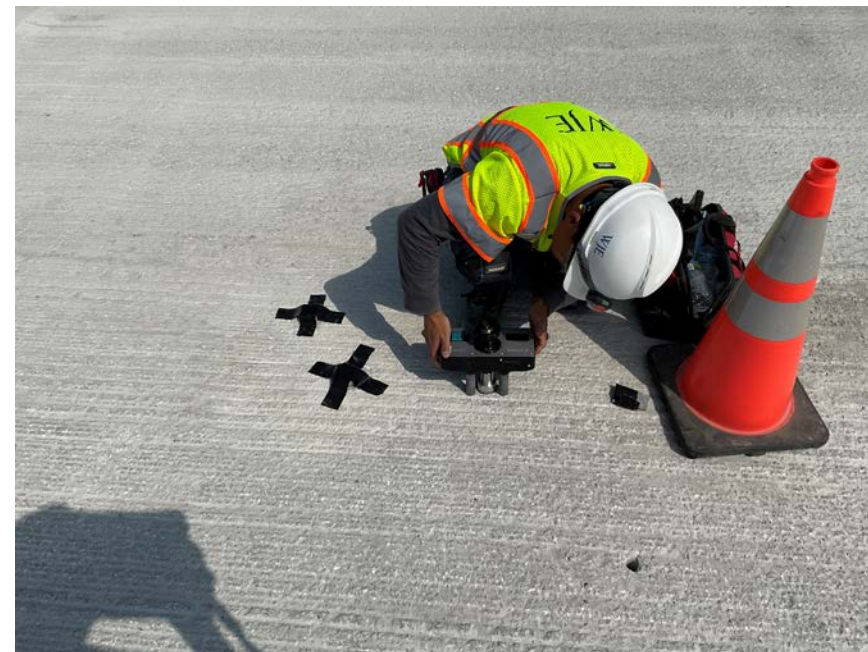
➤ Bond-testing of existing overlay to remain
