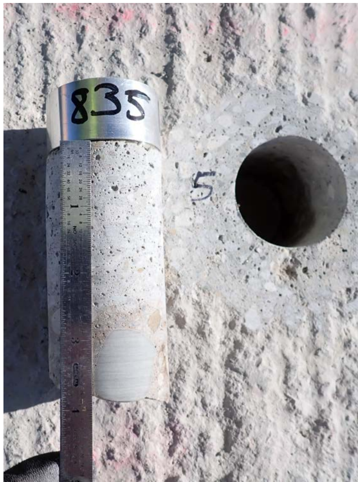
➤ Bond-testing of existing overlay to remain
