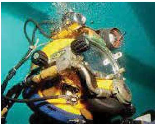
Fig. 10: Diver's helmet contains air, communications, video, and lighting
