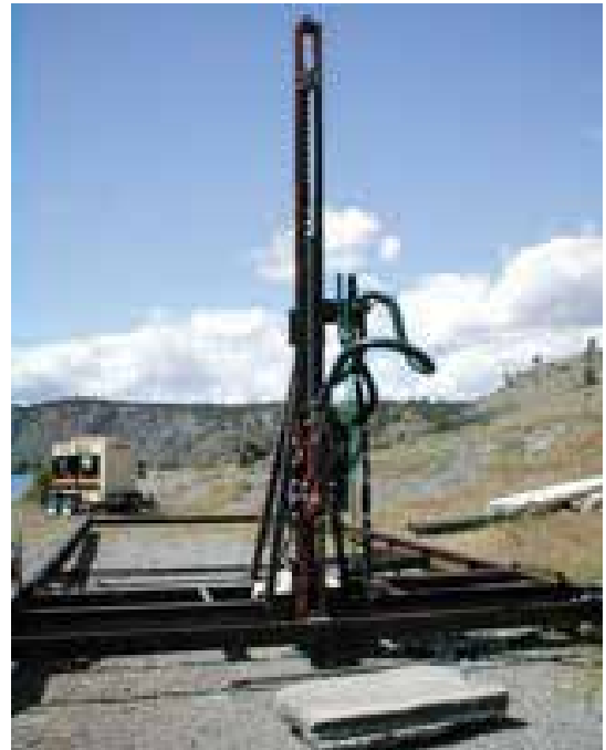
Fig. 12: Custom 2-1/2 in x 37 in (64 mm x 940 mm) deep hydraulic percussion drill for rock anchors
