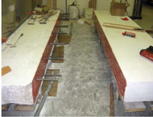
Larger section being fabricated from smaller marble pieces
