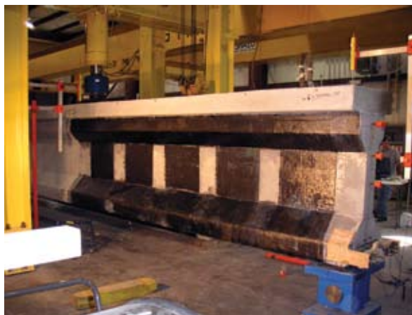
Load testing of AASHTO girders in lab
