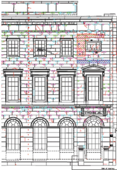
Thermography output showing areas of moisture retention within the stone and heat loss around the windows as well as locations of previous repairs
