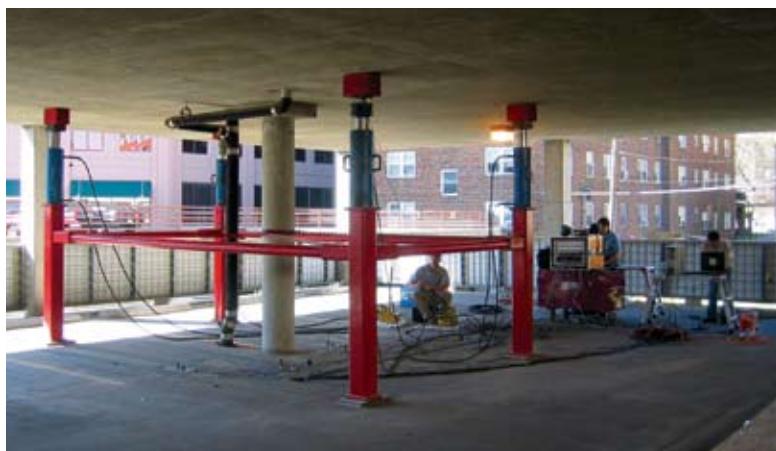
Fig. 1: Load testing of slab using hydraulic jacks and steel frame to apply the loads. Note the computers acquiring data
