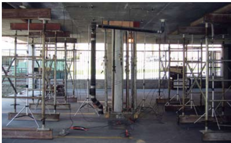
Fig. 2: Underside of test slab showing sensors during load test of Option 2. Shoring was used as a safety measure (it was not in contact with the slab bottom)
