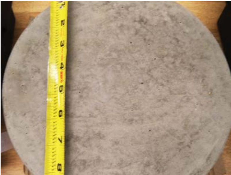
Fig. 6: Concrete specimen surface with a light steel-troweled finish
