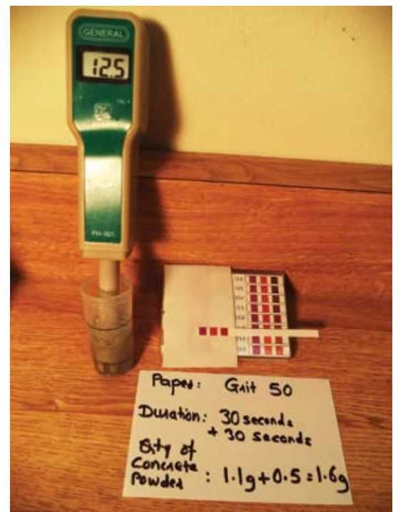
Fig. 8: The pH of a concrete powder sample obtained after 60 seconds of surface sanding using 50-grit sandpaper revealed pH of 12 using pH strip and 12.5 using pH meter
