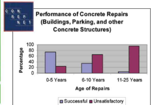
Fig. 3: Failure rate of repairs based on elapsed time since the repair was performed 3
