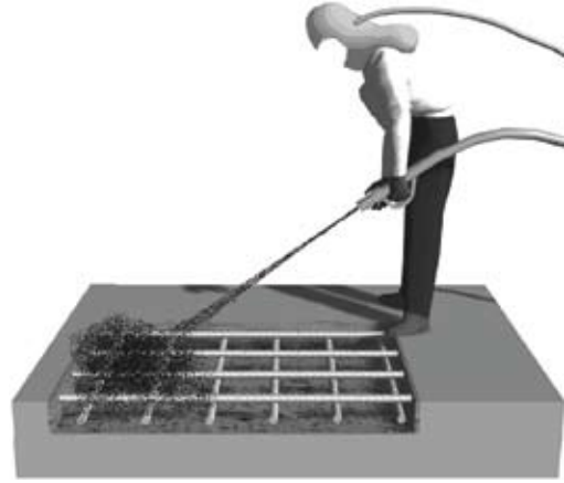
Fig. 7—Clean the exposed concrete and reinforcing bars with high-pressure water or abrasive blasting.
