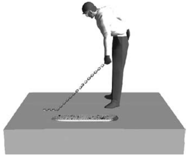
Fig. 1—Sound the concrete surface to locate delaminated areas. Chain drags can be used for sounding.
