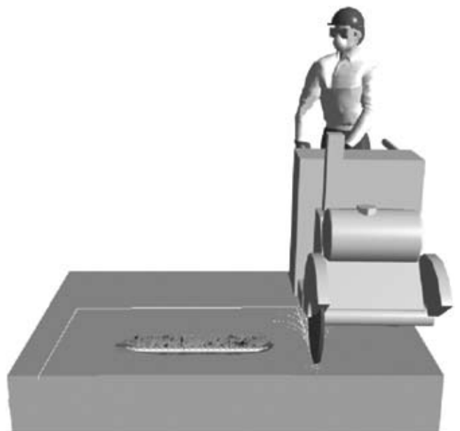
Fig. 3—Sawcut the repair perimeter, but no deeper than the thickness of the concrete cover over the reinforcement.
