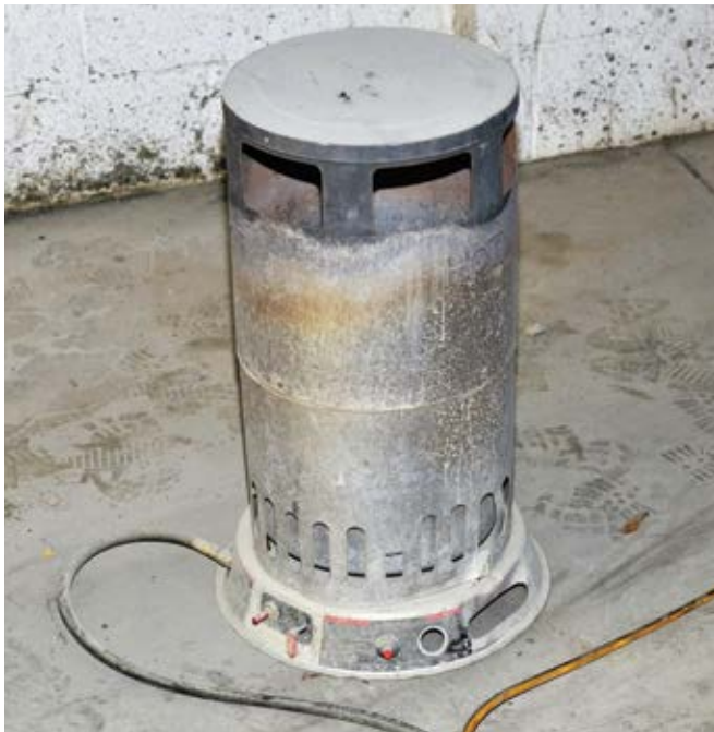
Fig. 1: A temporary heater is common on a construction site when working during cold weather
