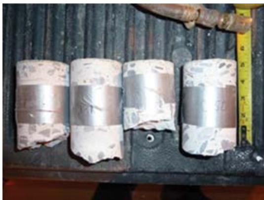
Fig. 3: Concrete cores for investigative testing
