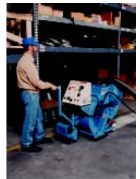
Shot blasting is one of the most common floor preparation methods.
