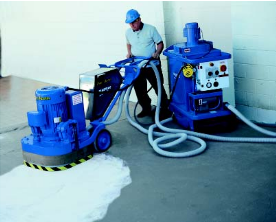
Diamond cutters/slicers are a relatively new method for removing thick coatings, mastics and polymers. Also used to level out surfaces, they leave a smooth, even finish.
