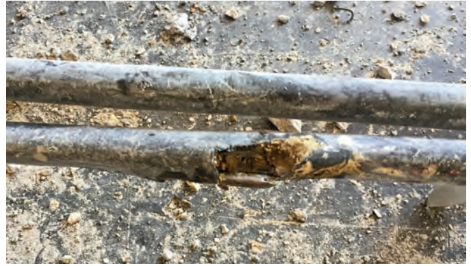
Fig. 10: Post-tension strand damage after slab removal
