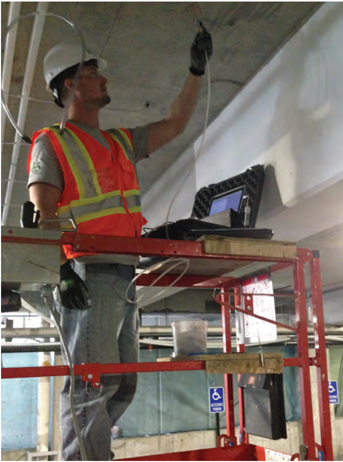
Fig. 6: Post-tension corrosion evaluation procedure (moisture test)
