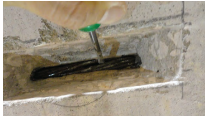
Fig. 3: Screwdriver penetration test detecting broken wires
