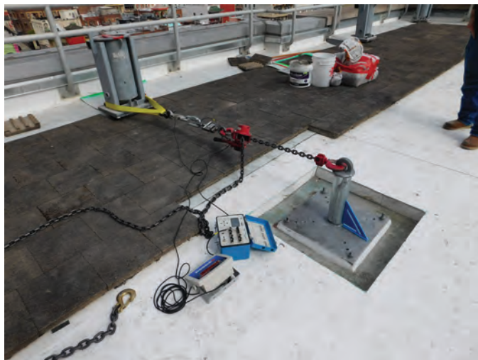
Fig. 5: Load test of fall arrest anchorage (right) reacting off a davit base (left)
