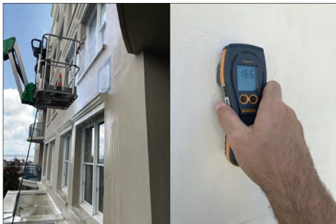
Fig. 5: Soak test on stucco façade (left) and radio frequency moisture testing (right)
