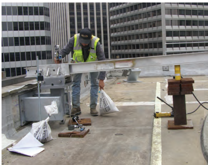
Fig. 6: Load test of davit pedestal replicating overturning moment generated during use
