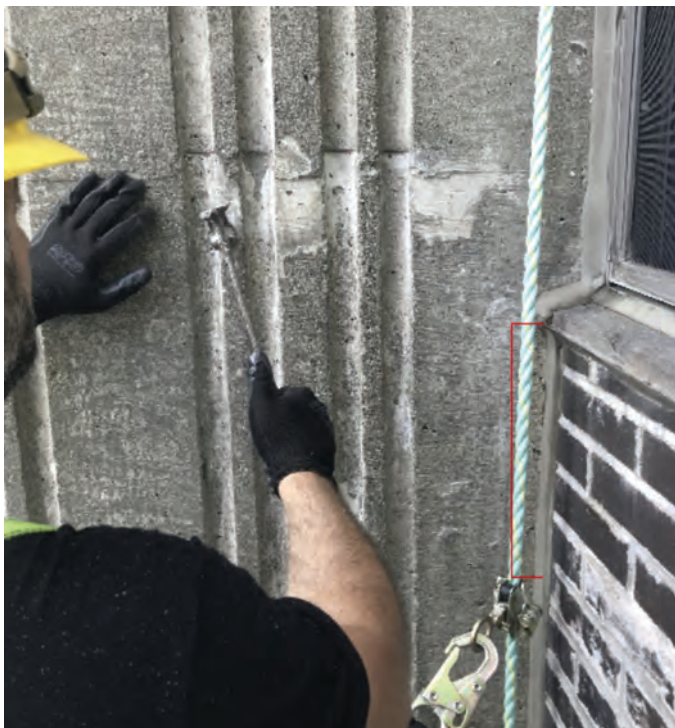
Fig. 3: False positive indication—lifeline detected as exposed rebar
