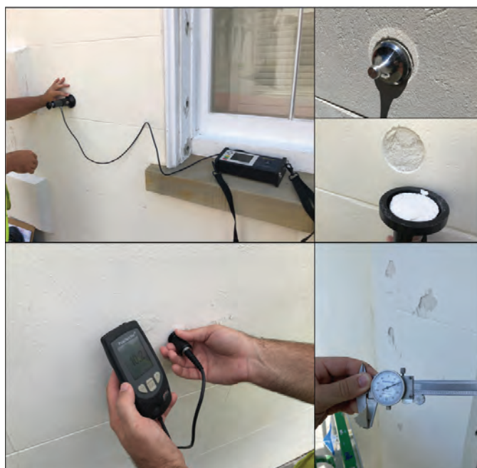
Fig. 10: Coating bond testing (top), ultrasonic thickness testing (lower left), and direct thickness testing (lower right)
