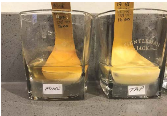
Fig. 4: Swelling waterstop being tested with shaft water vs tap water.
