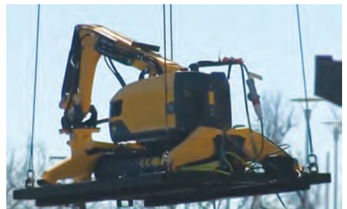
Fig. 4: Remote controlled robot used for roof demolition (photo courtesy of KCRA 3 News)
