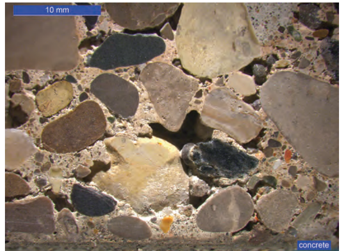
Fig. 7: Microscopic view of original concrete material
