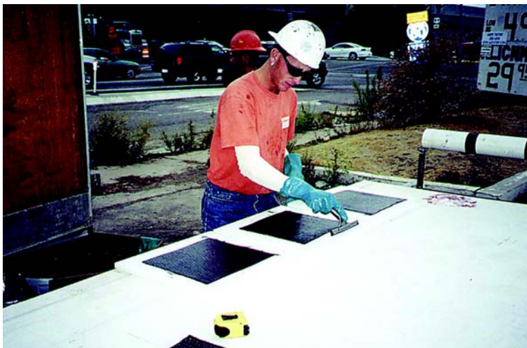
Preparing flat-panel specimens for QC testing
