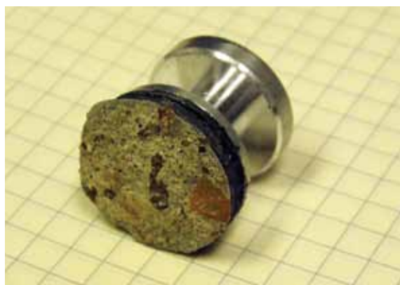
Fig. 7: Dolly showing cohesive failure of the concrete substrate
