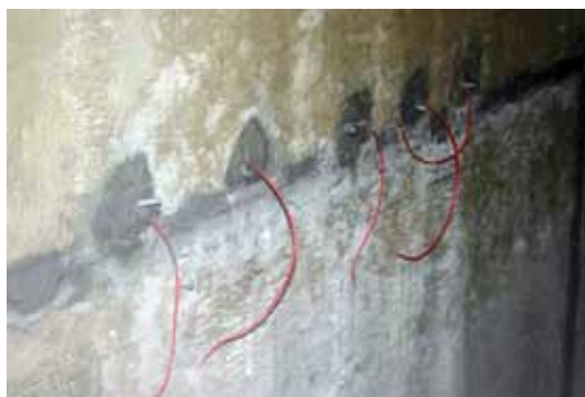
Reference electrodes set up for stray current testing
